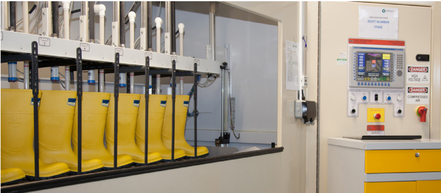
Dielectric boots under test at the Workmaster™ boot factory
